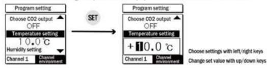
Operate Cooler relay when current temperature is higher than that of setting temperature
