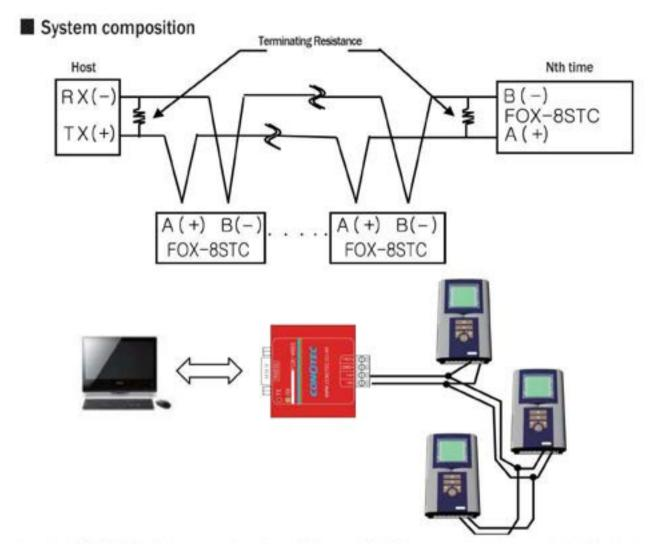
There is "RS485" for 1:N communication which uses RS 485 communications standard. At this time, the device will be SLAVE device. To communicate with PC program, additional RS485 to 232 Converter is needed. (Shall be purchased additionally)
