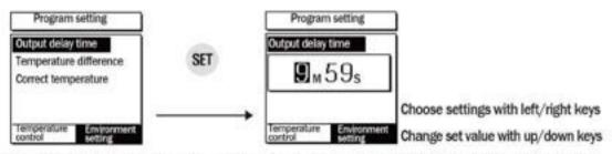
Use this function when there is a problem due to frequent use of ON/OFF operation by controlling targets such as a refrigerator and compressor.
