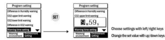
■ The buzzer will be ON during warning time and the buzzer will be OFF when setting the warning time as O second
