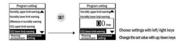
Setting a point that makes warning against low CO2 when current CO2 is lower than that of a certain CO2. Warning against low CO2: When current CO2 is lower than set value of CO2 lower limit (Buzzer ON). Lift after warning against low CO2: when current CO2 is higher than 'Set value of CO2 lower limit - Set value of difference in CO2 warning' (Buzzer OFF).
