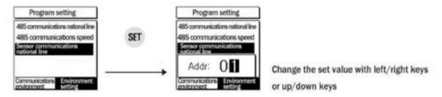
■ It is an ID that request measured values to FS-600R (Sensor) by making 8STC main host.
