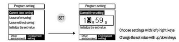
■ Change the time if the time in measuring screen is not consistent with the correct time
