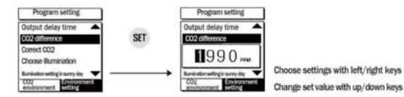
Certain interval is needed between ON and OFF for ON/OFF control (Set the interval between ON/OFF) If On and OFF are operated too often, relay or output contact will be worn rapidly or hunting (Chattering, Oscillation) will occur due to outside noise. To prevent these phenomenons, setting temperature difference to protect contact of equipment or others shall be needed.
