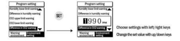
Set a hysteresis interval between warning ON and OFF. It will be applied to high CO2 warning as well as low CO2 warning
