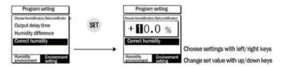
It is the function of matching the hygrometer of this product to other precision hygrometer if there is difference between these two hygrometers.
