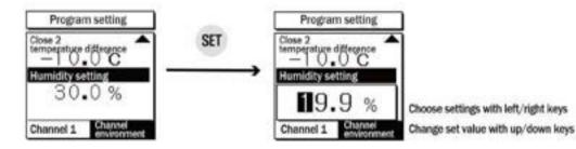
Operate when choosing humidification or current humidity is lower than setting humidity
