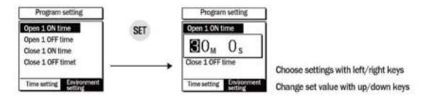
■ Open 1 phase control time: Open 1 ON time (Open operation ON)/ Open 1 OFF time (Open operation OFF) Close 1 phase control time: Close 1 ON time (Close operation ON)/Close 1 OFF time (Close operation OFF)
