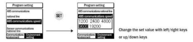
It is the communication speed for serial communications. It shall be in line with the HOST system and speed such as PC.
