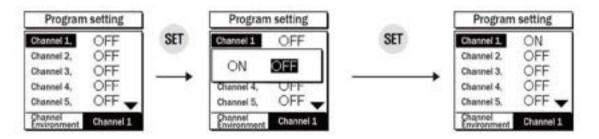
It can input 9 channels in maximum. It will moved to next channel when the user choose ON by channel.
