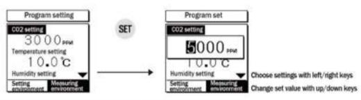
Operate when current CO2 is higher than that of set CO2.
