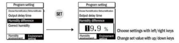
Certain interval is needed between ON and OFF for ON/OFF control (Set the interval between ON/OFF) If On and OFF are operated too often, relay or output contact will be worn rapidly or hunting (Chattering, Oscillation) will occur due to outside noise. To prevent these phenomenons, setting temperature difference to protect the contact of equipment or others shall be needed.
