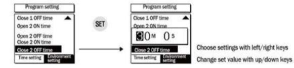
Open 2 phase control time: Open 2 ON time (Open operation ON)/ Open 2 OFF time (Open operation OFF)
