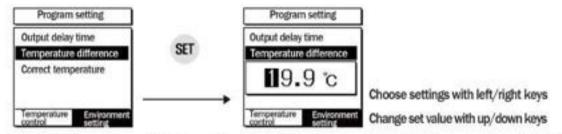
Certain interval is needed between On and OFF for On/OFF control (Set the interval between ON/OFF) If On and OFF are operated too often, relay or output contact will be worn rapidly or hunting (Chattering, Oscillation) will occur due to outside noise. To prevent these phenomenons, setting temperature difference to protect contact of equipment or others shall be needed.
