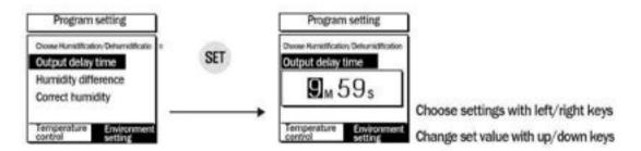
Use this function when there is a problem due to frequent use of ON/OFF operation by controlling targets such as a refrigerator and compressor.
