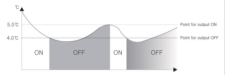
Setting Temperature 5.0°C, Temperature Deviation: 1.0°C Current Temperature > Setting Temperature + Temperature Deviation → Output ON Current Temperature ≤ Setting Temperature → Output OFF
