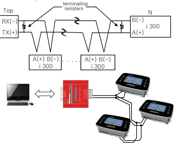
"RS485" for 1:N communication is available that uses the RS485 communication standard. At this time, the device becomes a slave. A separate RS485 to 232 converter is necessary to communicate with computer programs. (Sold separately) Communication cable should be twist pair cable suitable for RS485 communication.
