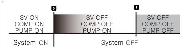
E.g.) Suppose stop delay time is 60 seconds, the system is turned OFF at and the output of the SV/COMP in operation will be turned OFF.
